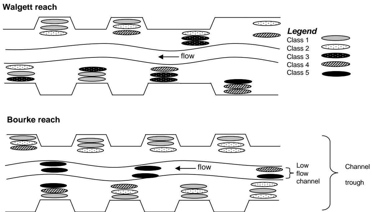
**Fig. 6** The mosaic of sediment textural classes along the two reaches in the study area.
