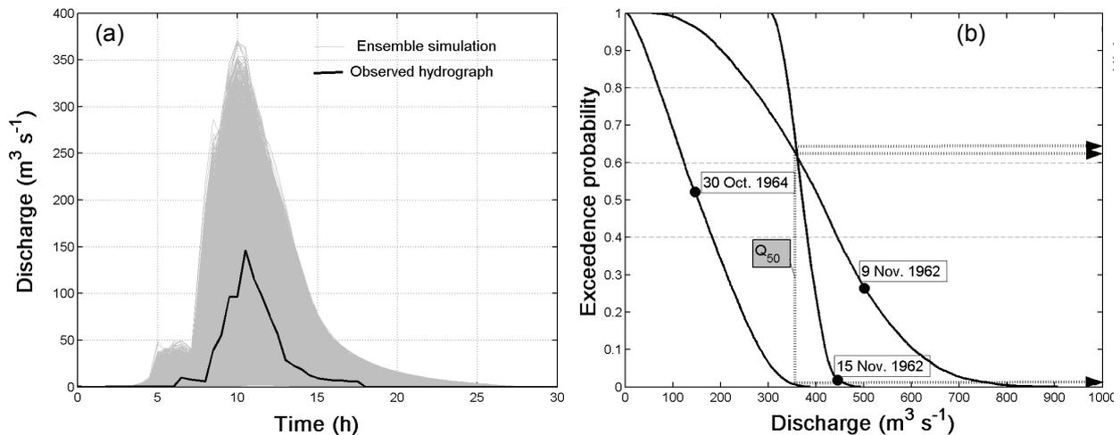
**Fig. 4** (a) Example of ensemble simulation along with the observed hydrograph for the 30 October 1964 event of the Esaro River. (b) Peak flow exceedence probability distribution (solid black line) obtained for three events occurred for the Esaro River, along with the observed peak flow magnitude (black dots) and the  $Q_{50}$  value.
