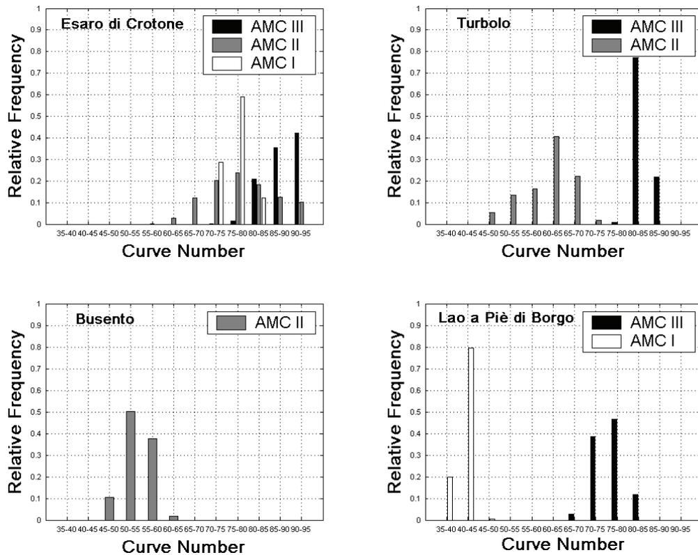
**Fig. 3** Histograms of relative frequency distribution of the *CN* parameter obtained for the gauged sites from the ensemble members that have a peak flow magnitude between  $\pm 20\%$  of the observed one.
