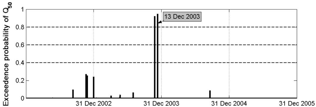
**Fig. 5** Time series of simulated exceedence probability of  $Q_{50}$  for the Valanidi basin and the mark of the date of occurrence of a documented severe flood event.
