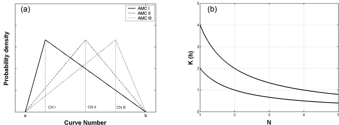
**Fig. 1** (a) Effect of antecedent moisture condition on the location and shape of the  $CN$  probability distribution; (b) example of the limits defining the acceptable region in the IUH parameters space.
