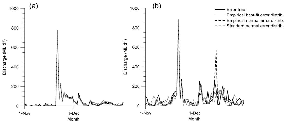
Fig. 3 Comparison of daily end-of-system flows, November–December 2003. (a) IQQM with channel routing on links; (b) IQQM with all routing removed.
