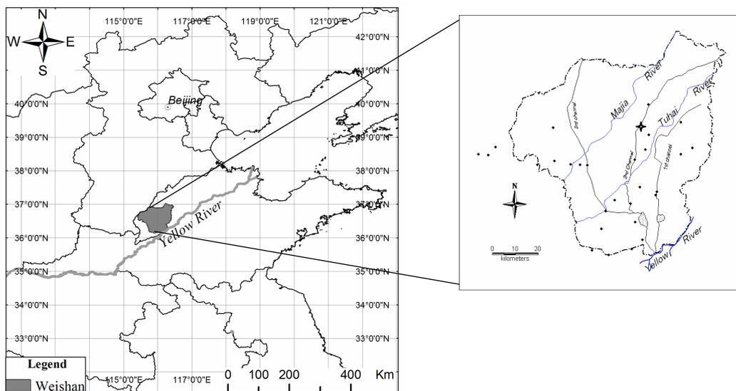
**Fig. 1** The Weishan irrigation district. The black points show survey sites and the star shows the position of the long-term gauging station at Gaoying.
