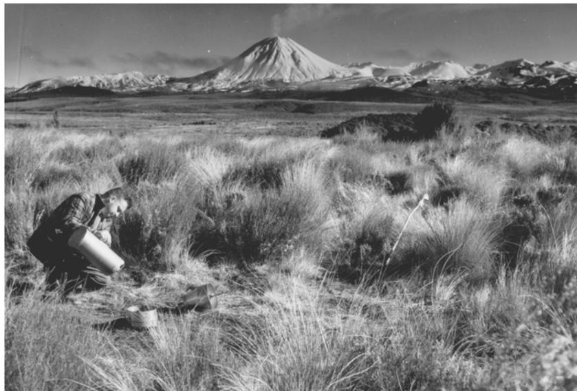
**Plate 3.1** Storage raingauge in the Tongariro basin, New Zealand.
