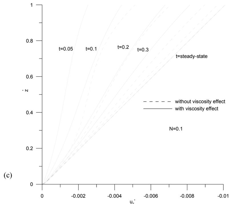
**Fig. 3** The predicted soil displacements versus dimensionless vertical depth for  $K^* = G^* = \lambda^* = 1$  and  $h_1/B = h_2/B = 0.01$  at various dimensionless times when  $N = 0.001$ , 0.01, and 0.1.
