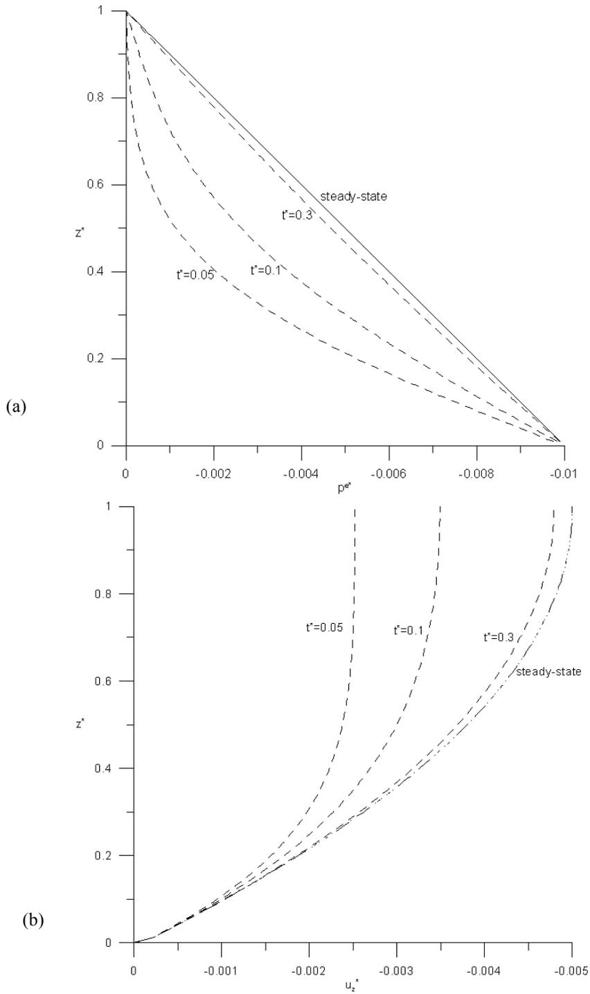
**Fig. 2** The simulated results for (a) excess pore water pressure and (b) soil displacement at different dimensionless time for  $G^* = N = 0$ ,  $K^* = \lambda^* = 1$ ,  $h_2/B = 0.01$  and  $h_1 = 0$ .
