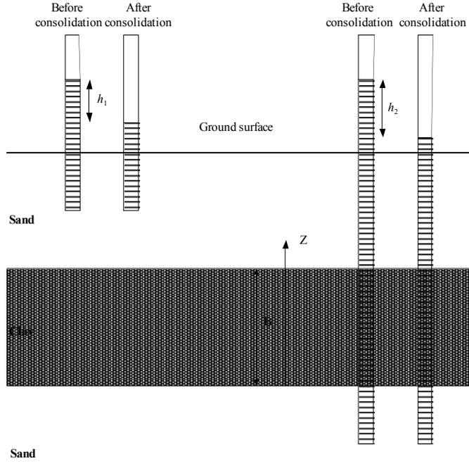
**Fig. 1** Schematic diagram of soil consolidation due to the change in groundwater level in response to the pumping in sandy aquifers (modified from Tsai, 2009).
