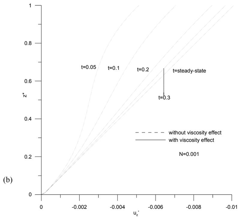
the viscosity effect is crucial and should be consider for consolidation in the clay layer when the adjacent aquifers are subject to a large pumping rate.
