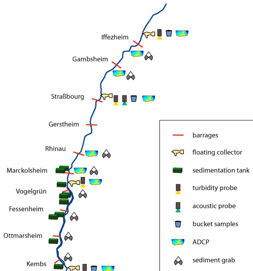
**Fig. 3** Impounded section of the Upper Rhine River. Sediment monitoring techniques.
