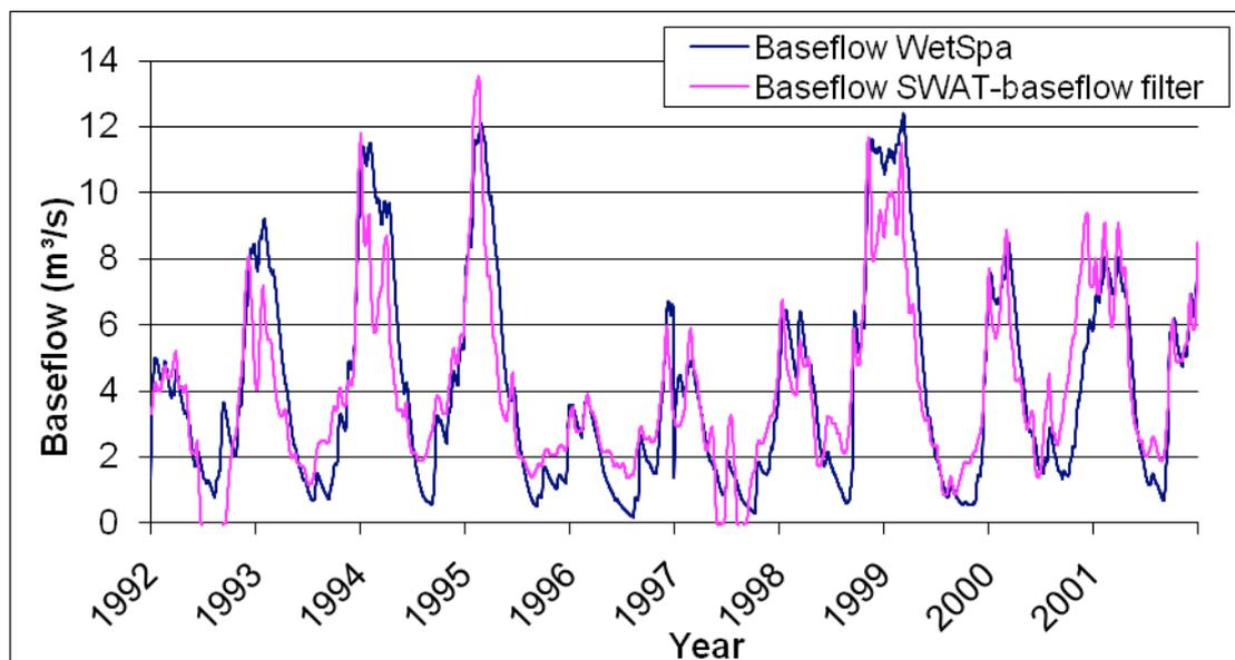
*Fig. 2 Comparing baseflow simulated with WetSpa and baseflow filtered by SWAT baseflow filter.*
