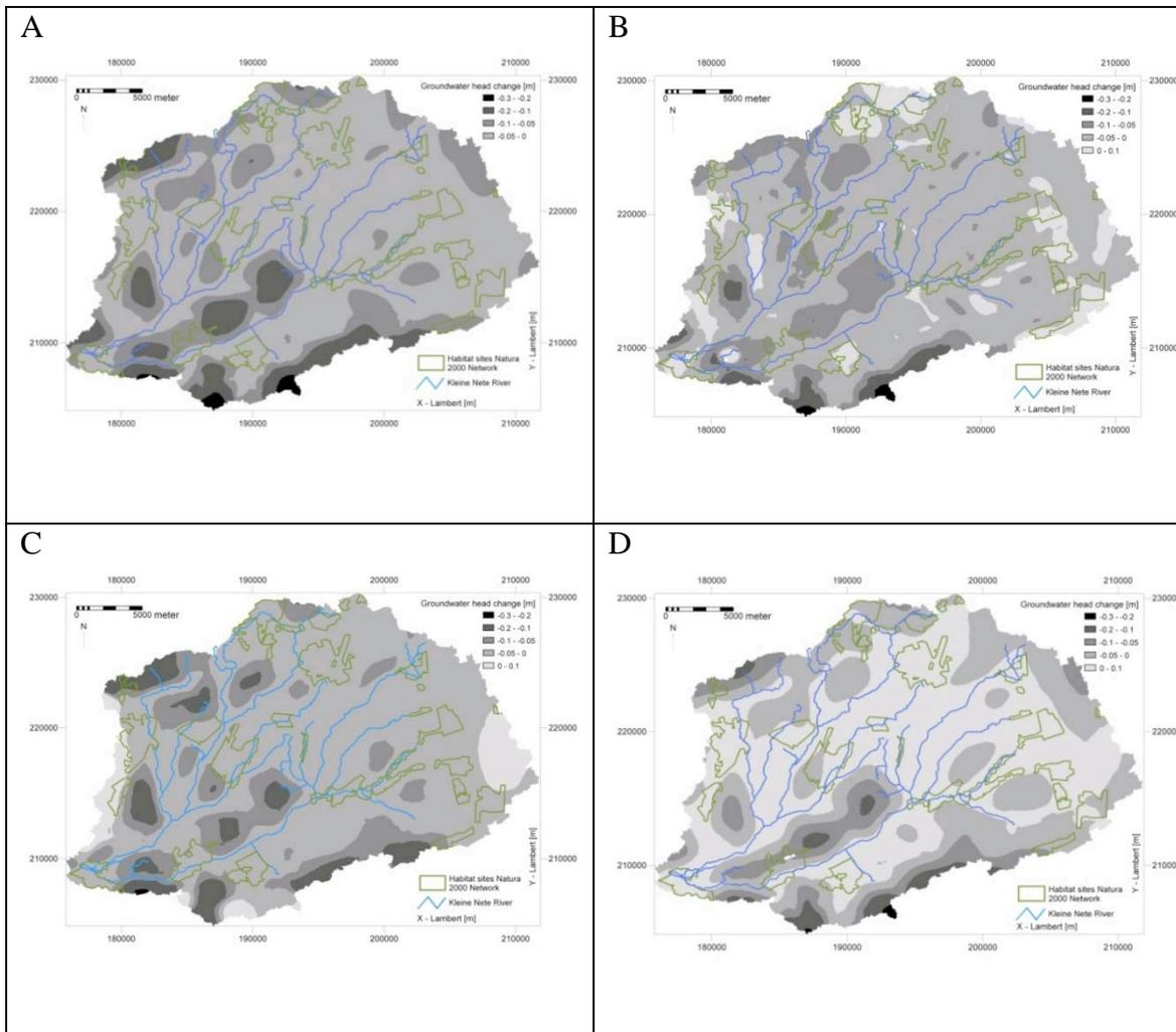
**Fig. 7** Change in average groundwater head (a), MHGL (b), MLGL (c) and MSGL (d) between the reference condition (1960-1991) and the average of the twenty-eight scenarios (2071-2100).
