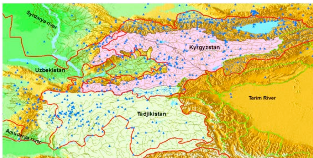
Fig. 1 Points of observation on precipitation and air temperature (blue triangles), red lines – state boundaries. Pink color – Syrdarya basin, light green – Amudarya basin.
