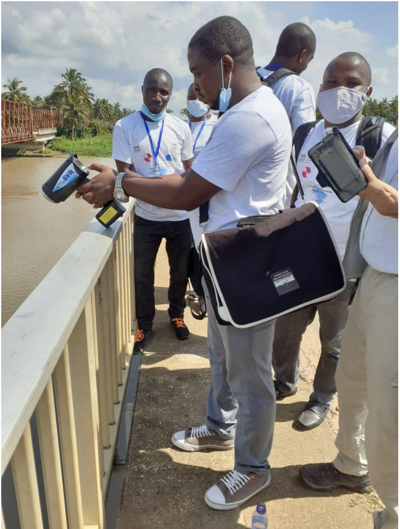
Picture 5: Measurement of the velocity of runoff using radar in the Mono River Bridge at Grand Popo.
