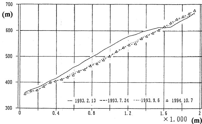
Fig. 7 Change in the longitudinal profile of the Akamatsu-dani.
