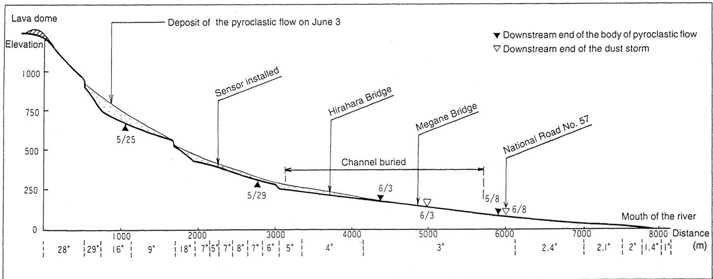
**Fig. 2** A longitudinal profile of the Mizunashi River showing the deposition associated with the pyroclastic flows which occurred on 3 June and 8 June 1991 (produced by the Erosion Control Department, Public Works Research Institute, Ministry of Construction).
