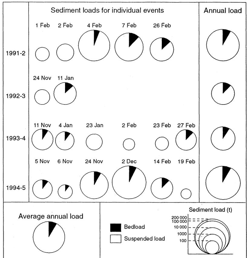
**Fig. 3** Flood-by-flood and annual variation in total sediment loads showing the proportion of bed load and suspended load. Note the logarithmic scale.
