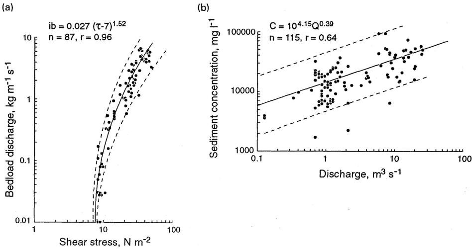
**Fig. 2** Bed load (a) and suspended load (b) rating curves for Nahal Eshtemoa. The pecked lines represent the 95% confidence intervals of the regression lines. In both instances, the relations have been adjusted for the statistical bias introduced by the log-log transformation of the variables (Ferguson, 1986). *n* is the number of paired observations, *r* is the correlation coefficient.
