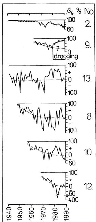
Fig. 2 The long-term course of the trap efficiency  $\beta_4$  of six selected reservoirs. Reservoirs are numbered as in Fig. 1.
