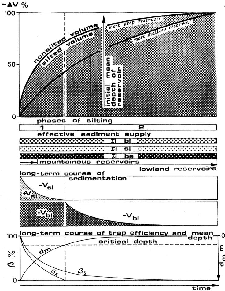
Fig. 3 Model illustrating the long-term course of reservoir silting: phases of silting: 1 = first, 2 = second; effective sediment supply:  $\Sigma l bl$  = bed load;  $\Sigma l sl$  = suspended load;  $\Sigma l be$  = material from bank erosion;  $+V_{sl}$  = retention of suspended matter;  $-V_{sl}$  = outflow of suspended matter,  $+V_{bl}$  = retention of bed load;  $-V_{bl}$  = outflow of bed load;  $d_m$  = mean depth of reservoir. For explanations  $\beta_4$  and  $\beta_5$ , see the text.
