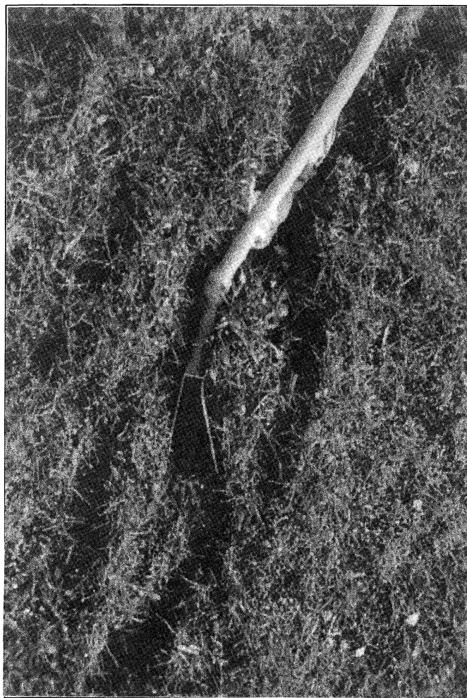
Fig. 2 Overland-flow sampler in measuring position, seen from above. The tube leading to the collecting bottle is shown.
