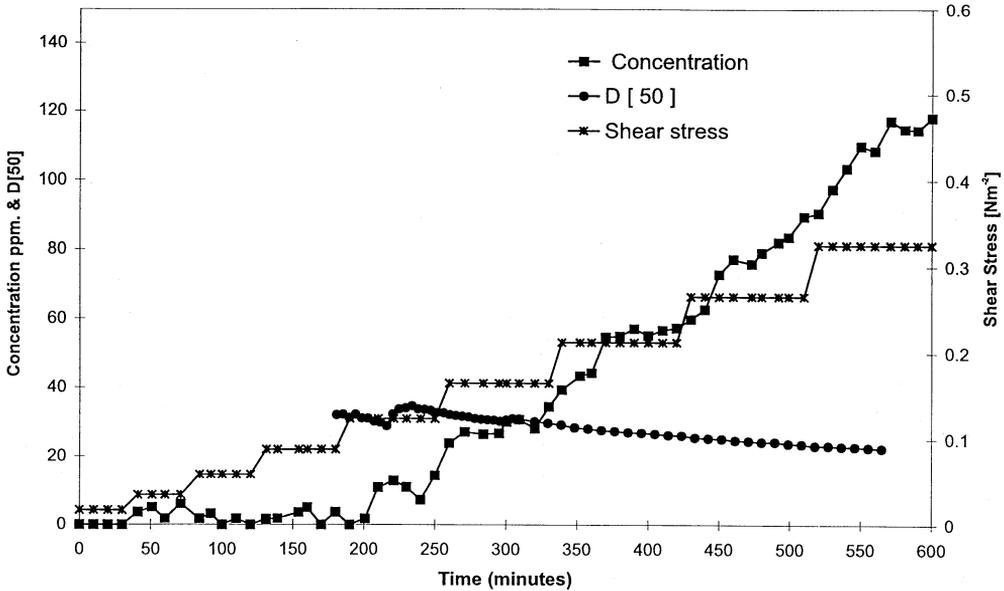
Fig. 4 Concentration, shear stress and median size vs time.
