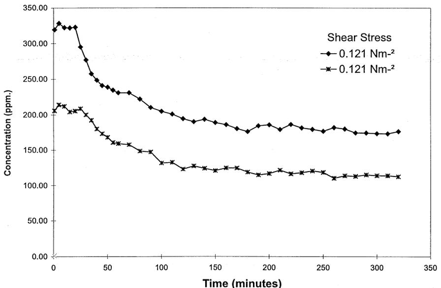
Fig. 2 Sediment concentration vs time, shear stress =  $0.121 \text{ N m}^{-2}$ .
