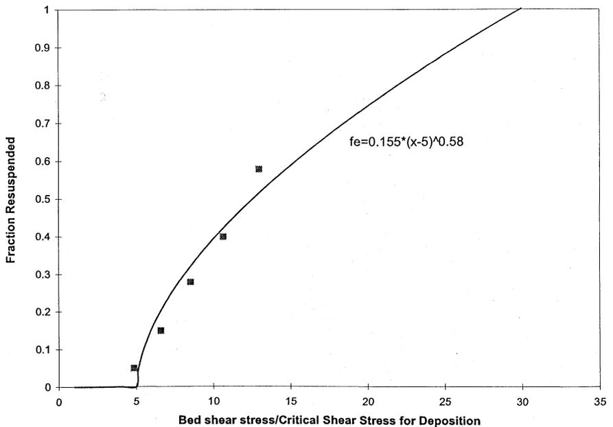
Fig. 6 Erosion function.
