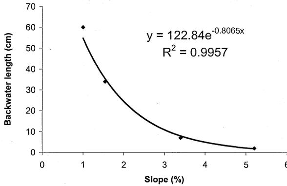
Fig. 3 Effect of slope on the length of backwater for medium nail density.
