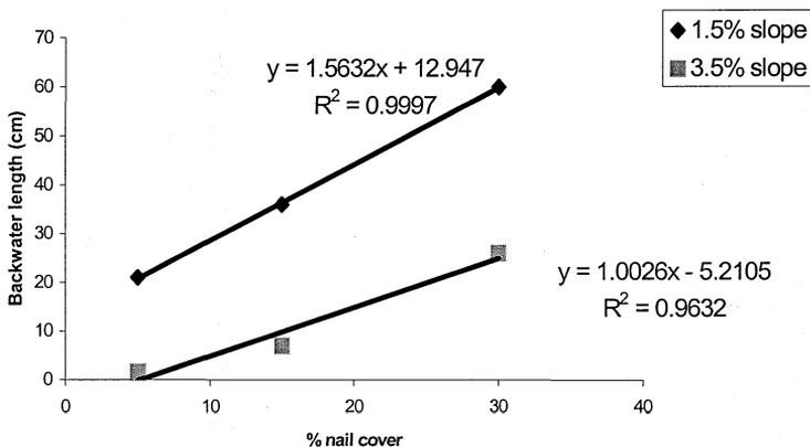
Fig. 4 Effect of nail density on the length of backwater on constant slopes.
