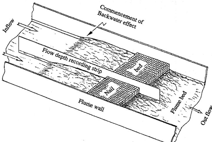
Fig. 1 Flume showing the position of buffer strip and flow height recorder.
