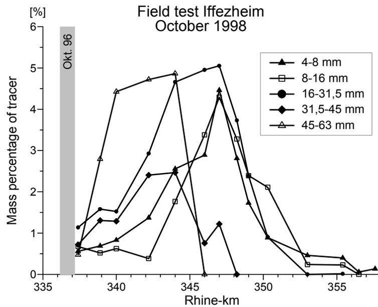
Fig. 3 Longitudinal tracer distribution 24 months after dumping.
