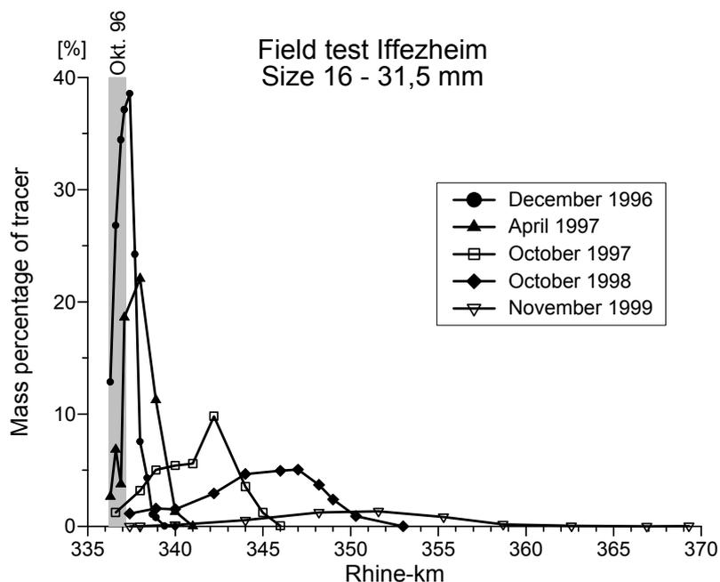
Fig. 5 Longitudinal dispersion of fraction 16–31.5 mm.
