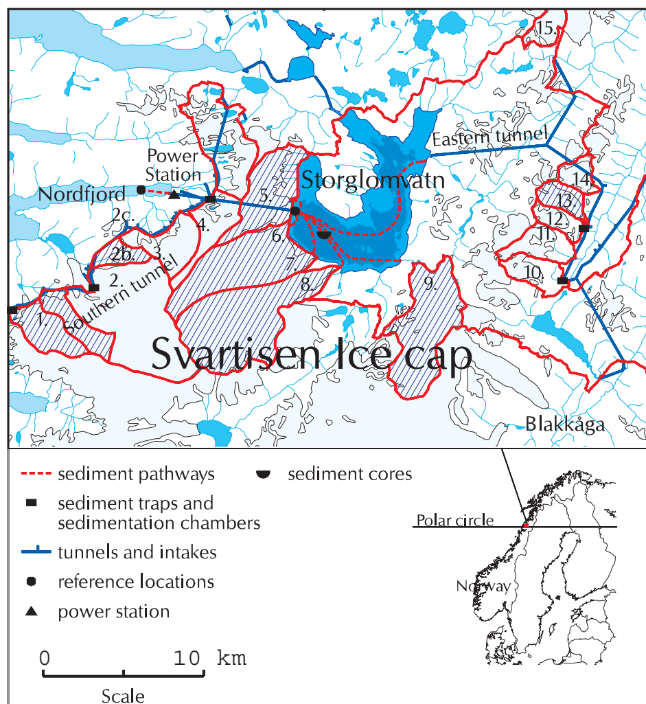
Fig. 4 Diversion tunnels and intakes of the Svartisen power plant. The sediment yield for some glaciers (cross-hatched) had to be estimated. The other numbered glaciers have been subject to direct measurements of sediment yield. Names of glaciers in Table 1. The sediment pathways refer to those used in the routing model.
