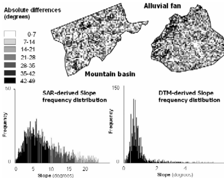
**Fig. 5** Upper: Absolute differences between the DTM and SAR-derived slopes for the mountainous (left) and the alluvial fan (right) portions of the basin. Lower: Frequency distributions of the DTM and SAR-derived slopes for the entire basin.
