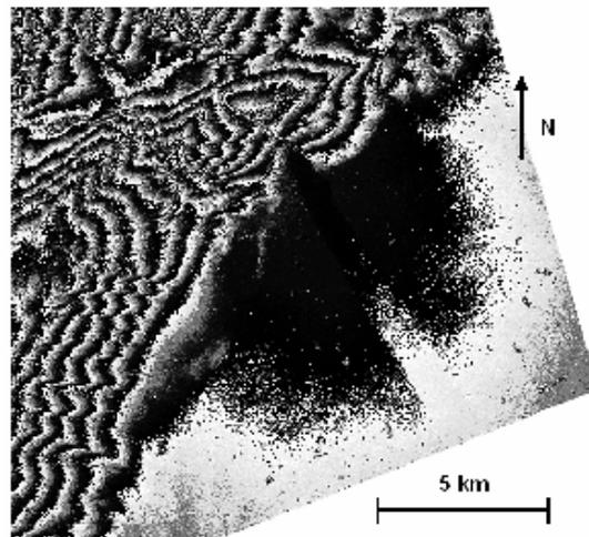
**Fig. 3** Georeferenced interferogram of the study area obtained from two ERS 1/2 SAR images. The alluvial fan shape can be recognized in the fringe pattern.
