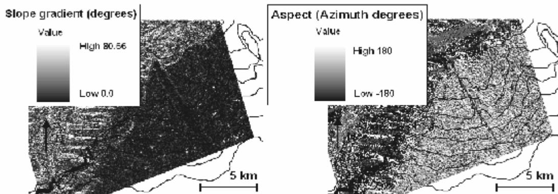
**Fig. 4** SAR-derived slope and aspect of the alluvial fan.
