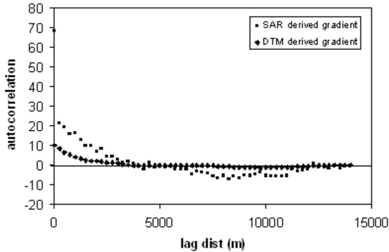
Fig. 6 Autocorrelation for SAR and DTM-derived slopes.
