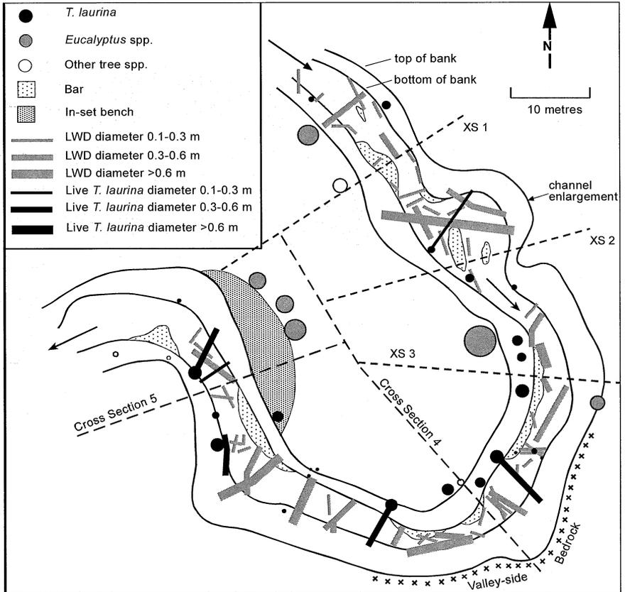
**Fig. 2** Location of trees and large woody debris in a sub-reach of Bruce's Creek. Circles represent tree diameters at breast height exaggerated by a factor of two.
