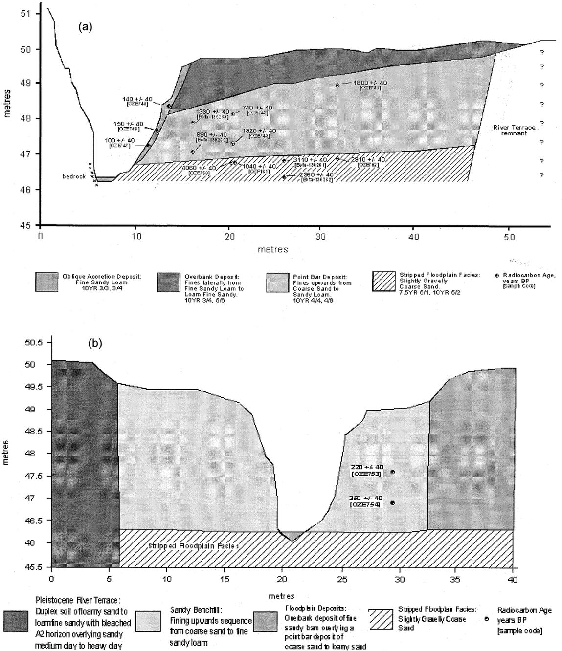
Fig. 3 (a) Flood plain stratigraphy at cross-section 4, and (b) flood plain and inset bench stratigraphy at cross-section 5.
