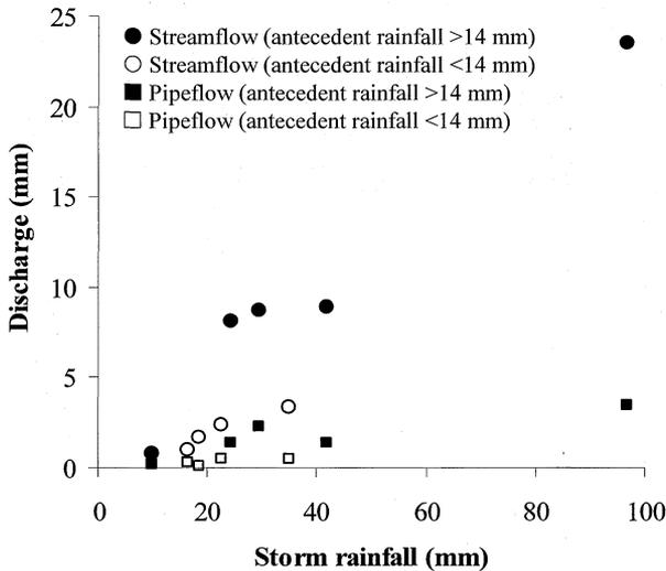
Fig. 3 Scatter plot showing the effect of antecedent rainfall (in the 3 days prior to the storm) on the relationship between storm rainfall and streamflow and pipeflow discharge.
