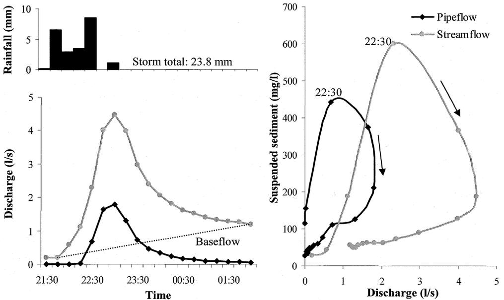
**Fig. 2** Streamflow and pipeflow storm hydrographs and suspended sediment hysteresis responses to rainfall on 10 January 2003.
