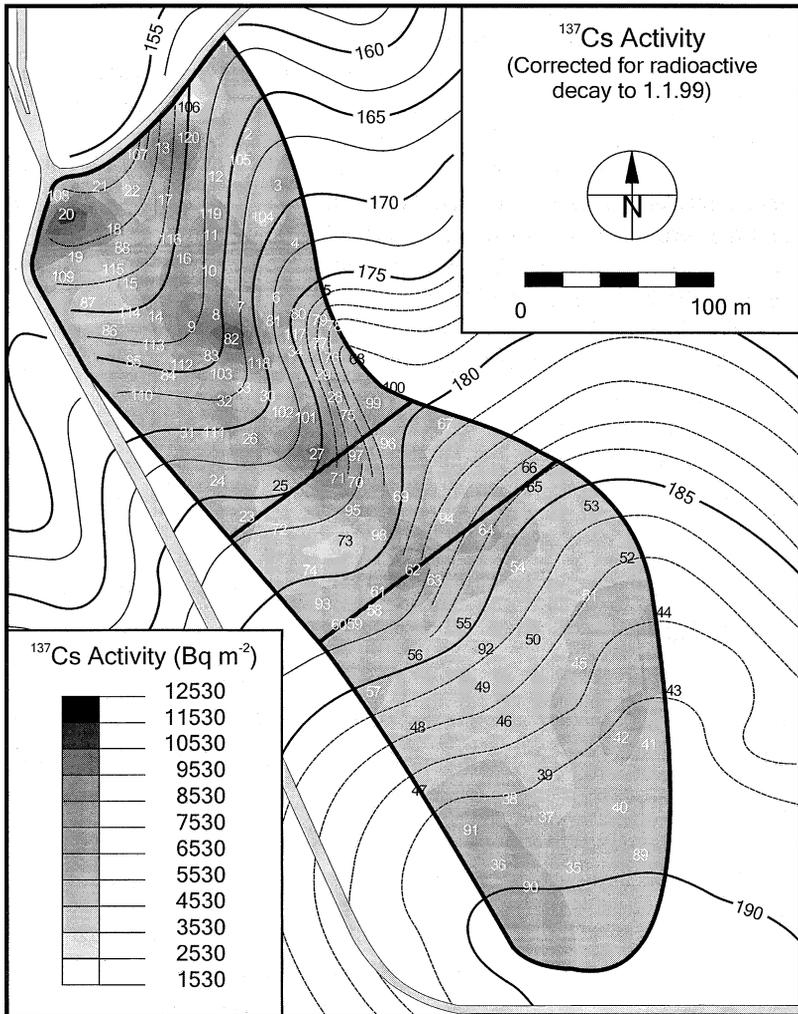
**Fig. 2** Distribution of <sup>137</sup>Cs activity in Auf dem Scheid. Sample points are numbered. Intervals were chosen to indicate areas with values greater and smaller than the reference inventory of 5530 Bq m<sup>-2</sup>.
