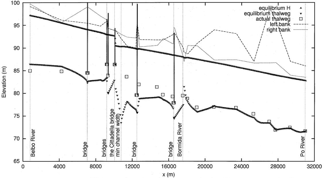
Fig. 3 Equilibrium configuration of bed topography for 100 years water and sediment discharge considering the actual geometry of the cross-sections.
