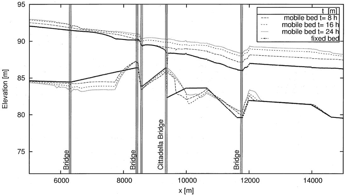
Fig. 4 Unsteady simulation: bed topography evolution during the increasing phase of an intense flood event.
