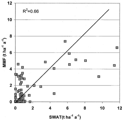
**Fig. 2** Comparison of calculated soil loss ( $\text{t ha}^{-1} \text{year}^{-1}$ ) using SWAT and MMF for 73 sub-basins of the Ybbs River basin.
