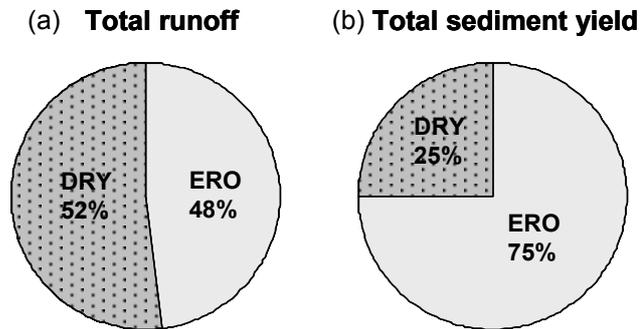
**Fig. 10** Contribution of the DRY and ERO surface types for the event of 11 August 1998 to: (a) total runoff, and (b) total sediment yield (simulated by the model KINEROS2).
