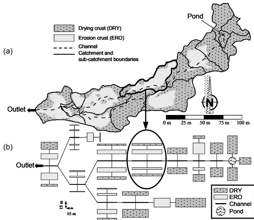
**Fig. 9** (a) Division of the Katchari catchment first into hydrological sub-units and then by taking into account the soil surface characteristics; and (b) representation of the catchment by a cascade of planes and channels for the KINEROS2 model.
