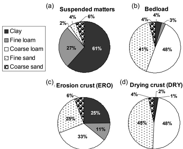
**Fig. 6** Grain-size distribution of suspended-matter, bedload, ERO and DRY soil surface types.
