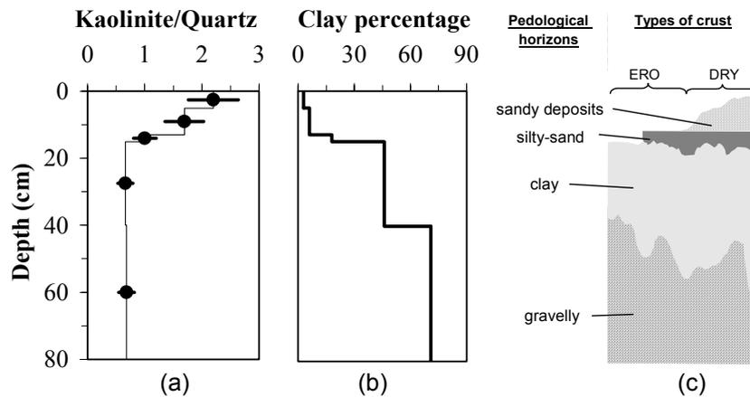
**Fig. 7** Vertical distribution of: (a) kaolinite/quartz ratio, (b) clay percentage (%), and (c) pedological horizons of a representative profile (from Karambiri *et al.*, 2003).
