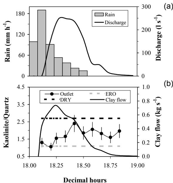
**Fig. 8** Storm event of 11 August 1998: (a) hyetograph and hydrograph; (b) kaolinite/quartz ratio and clay flow of the suspended sediment collected at the catchment outlet, kaolinite/quartz ratio of the erosion (ERO) and the drying (DRY) crusts (from Karambiri *et al.*, 2003).
