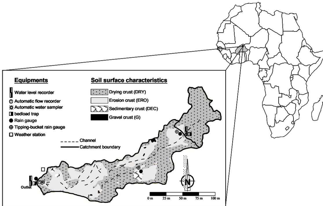
Fig. 1 Location, soil surface types and the equipment in the Katchari catchment.
