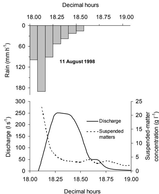
**Fig. 5** Behaviour of suspended-matter during a typical annual rainfall-runoff event.
