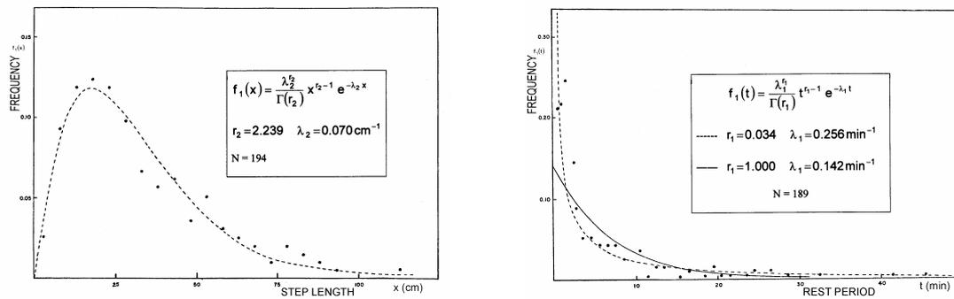
Fig. 6 Step length and rest period frequencies for a liquid discharge of 20 l s<sup>-1</sup>.
