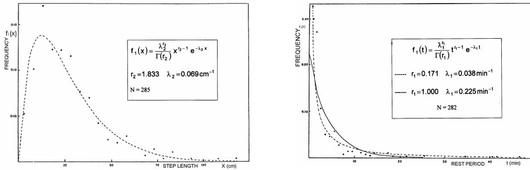
Fig. 5 Step length and rest period frequencies for a liquid discharge of 12 l s<sup>-1</sup>.
