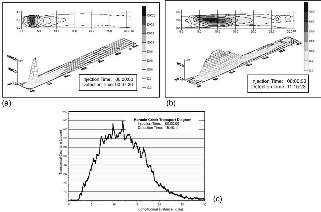
**Fig. 4** Isocount curves and 3-D representation. First experiment with  $^{198}\text{Au}$ : (a)  $t = 0.13$  h; (b)  $t = 11.26$  h; (c) example of transport diagram of the Horácio Creek,  $t = 15.80$  h.
