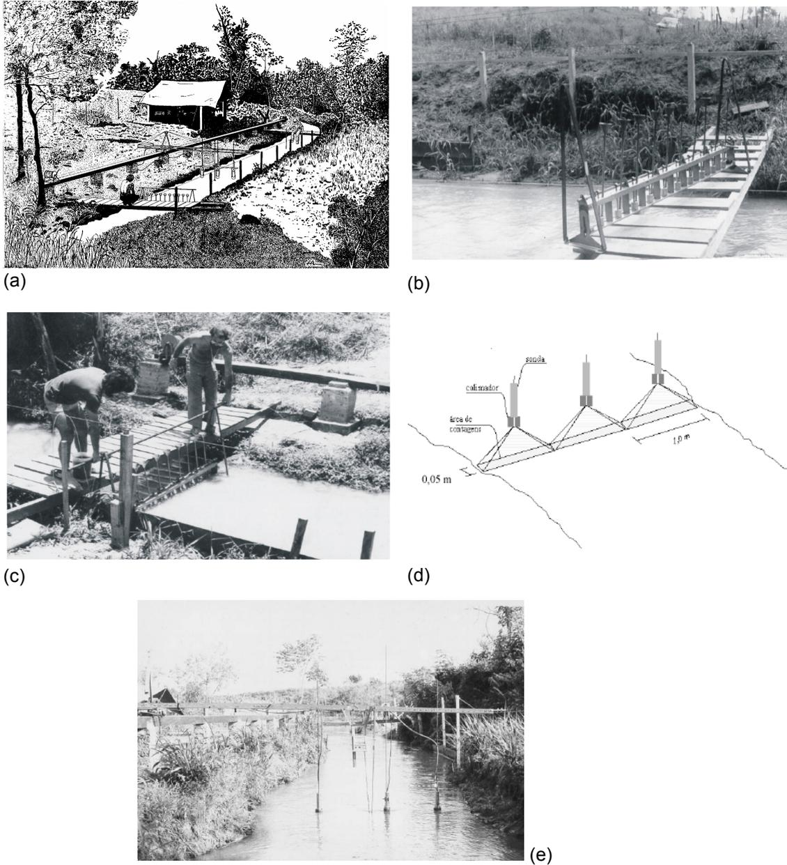
**Fig. 3** (a) Measurement stretch of the Horácio Creek. (b) Radioactive sediment injection equipment. (c) Radioactive sediments injection in Horácio Creek. (d) Areas covered by the radiation detectors. (e) Detection system used in the Horácio Creek.
