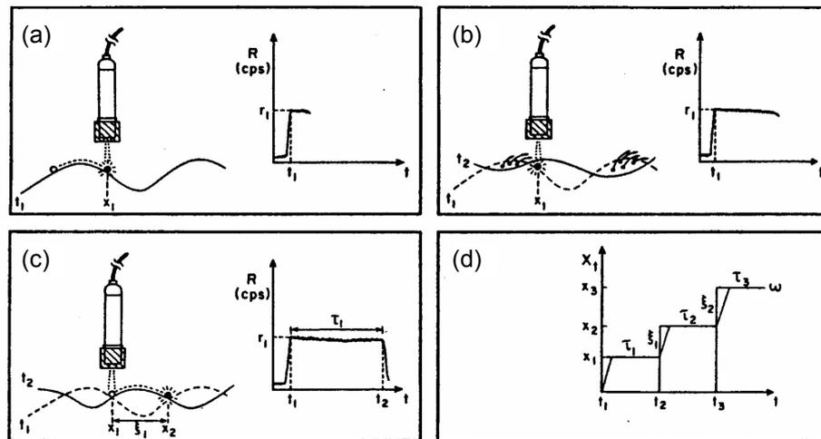
Fig. 2 Schematic diagram of step length and rest period measurements of single grains.
