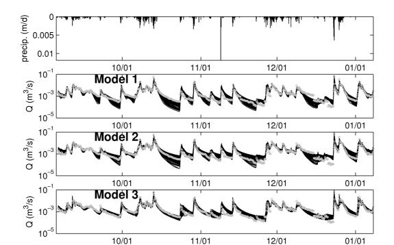
**Fig. 1** Simulation results for stream discharge. The Y axis is log transformed to outline more clearly model results at lower discharge. The calibration strategy focused on untransformed  $R_{eff}$ , and peak flows are correspondingly better captured. The plotted simulations are those found with Nash-Sutcliffe efficiencies over 0.75. Measured values are plotted as crosses.
