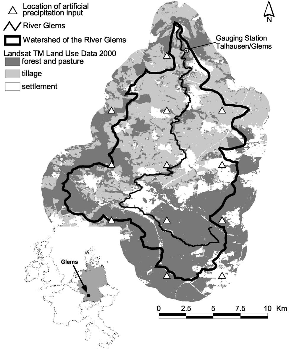
**Fig. 1** The watershed of the River Glems; land-use, location of the streamgauge and locations of artificial precipitation input.
