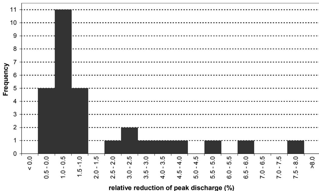
**Fig. 5** Frequency distribution of the relative reductions of peak discharges of yearly floods, as caused by changing soil management from 0% to 50% conservation tillage within the watershed of River Glems.
