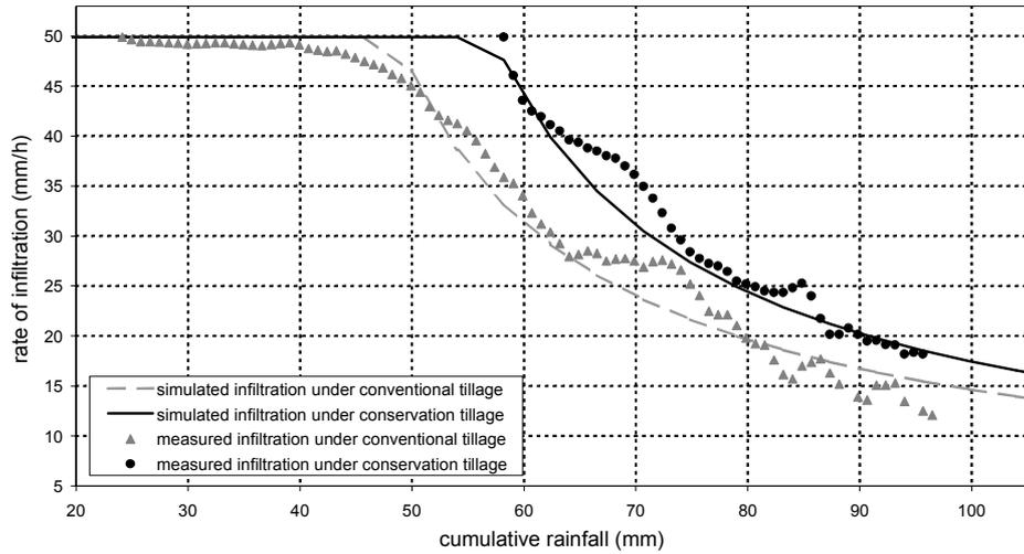
**Fig. 3** Numerical infiltration experiments with the infiltration module for a model soil under conventional and conservation tillage, along with experimental results from Gerlinger (1997).
