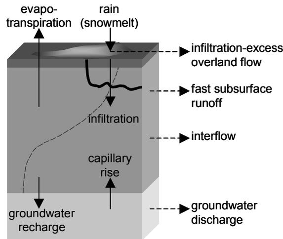
Fig. 2 Schematic sketch of the enhanced soil module of LARSIM.
