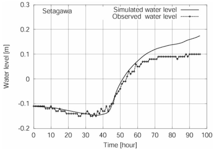
**Fig. 8** Simulated and observed water level of Lake Biwa.
