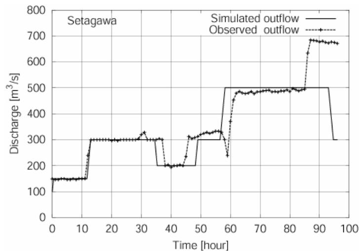
Fig. 7 Simulated and observed outflow at Seta weir.
