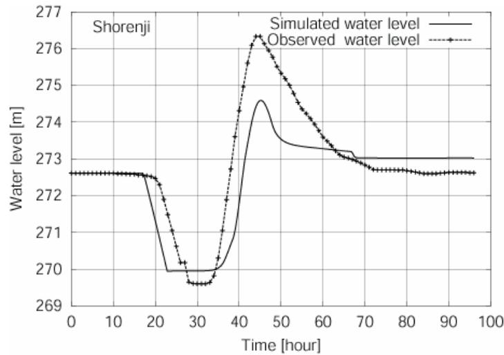
Fig. 6 Simulated and observed water level at Shorenji dam.
