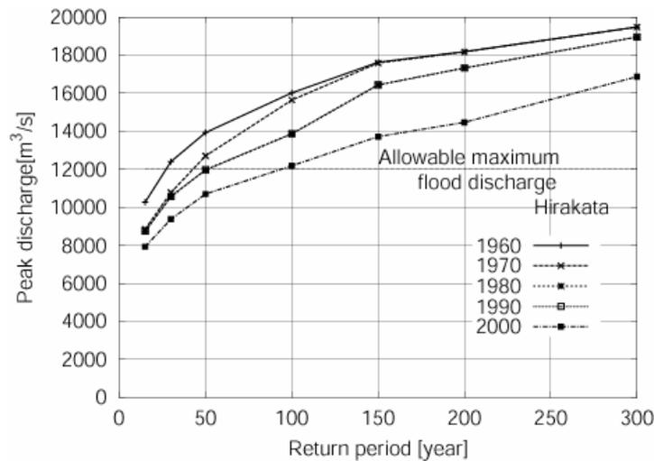
**Fig. 11** Simulated peak discharges at Hirakata with different magnitude of input rainfall. Years (1960, 1970, etc.) denote that the dams existed in the year are included in the simulation.
