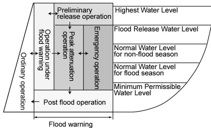
Fig. 3 Operation status and specific water levels of dam operation model.
