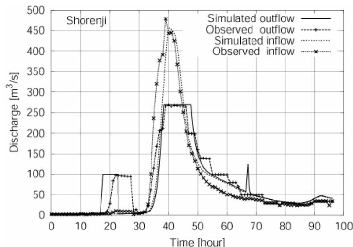
Fig. 5 Simulated and observed inflow and outflow at Shorenji dam.
