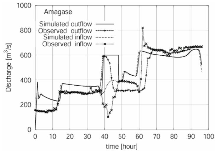
**Fig. 9** Simulated and observed inflow and outflow at Amagase dam.
