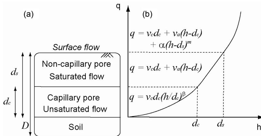
Fig. 2 Schematic diagram of the soil layer: (a) and stage–discharge relationship; (b) of saturated–unsaturated subsurface and surface runoff model.
