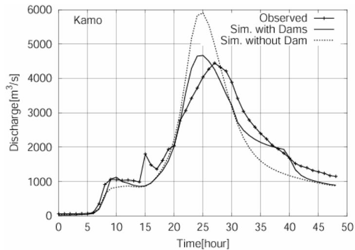
**Fig. 10** Simulated discharge (with and without dams) and observed discharge at Kamo.
