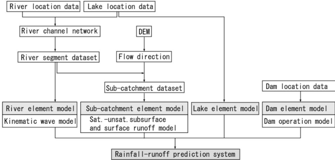
Fig. 1 Data processes and the whole structure of the system.
