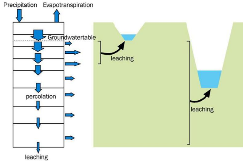
**Fig. 1** Illustration of the conceptualization of the water flow in SWAP (adapted from Schoumans & Silgram, 2003).
