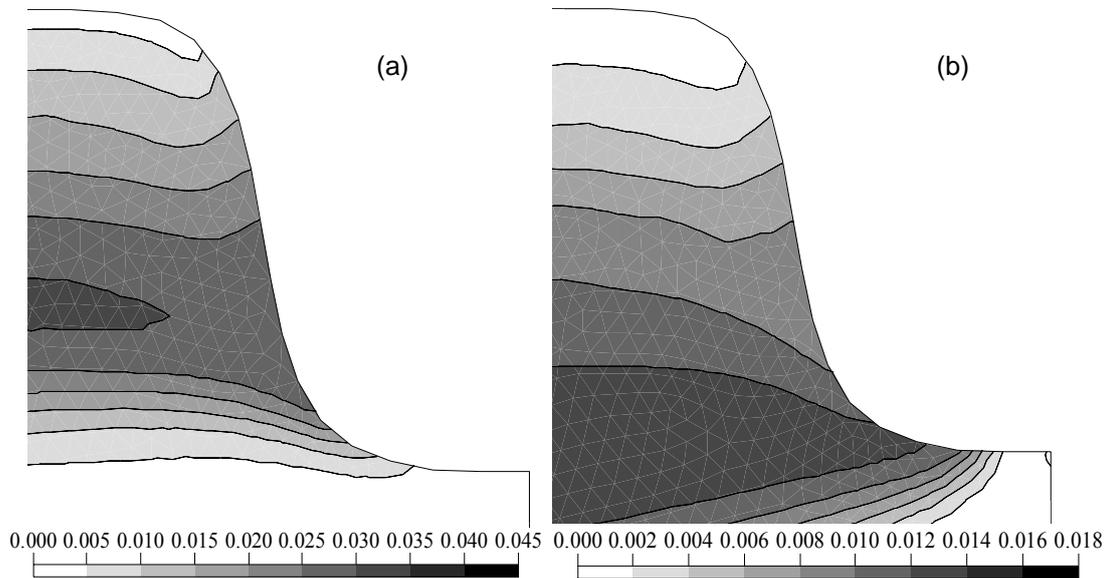
**Fig. 4** Distribution of the Cd-concentration ( $\mu\text{g cm}^{-3}$ ) close to the stream for the two time periods in Fig. 2: (a) winter in the years 5–6, and (b) winter in the years 27–28 (discharge occurs only through the stream bottom; area:  $1.1 \times 1.1$  m).
