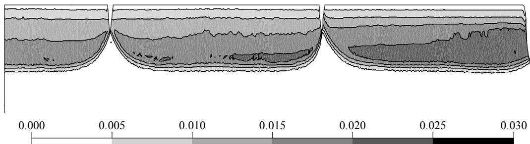
Fig. 6 Cd-concentration ( $\mu\text{g cm}^{-3}$ ) in a cross-section after 3118 days simulated using Hydrus-2D (stretching factor vertical coordinate: 5, width cross-section: 45 m).
