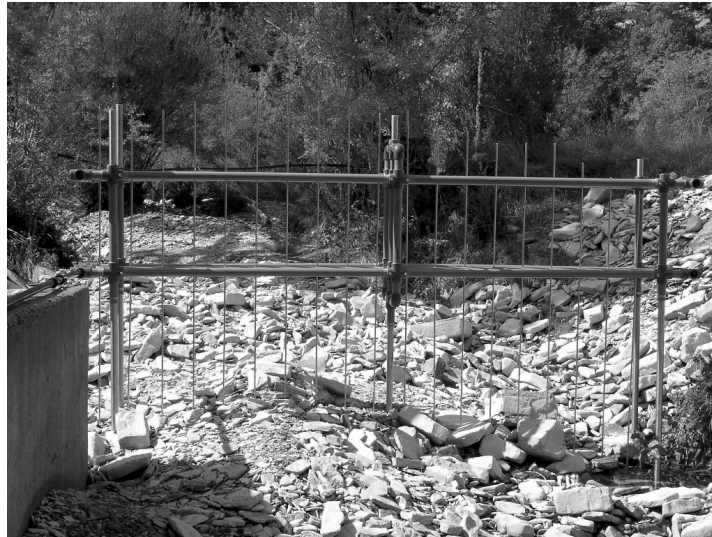
Fig. 2 View of the profilometer in the upper part of the gauging station. Note the coarse size of the accumulated material (September 2003).
