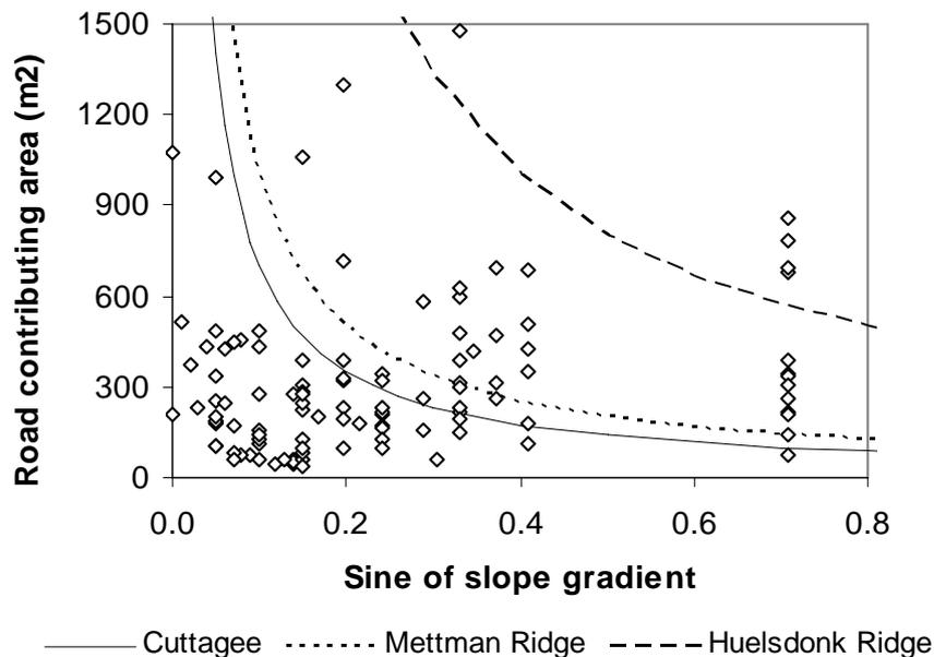
**Fig. 1** Contributing road area vs discharge hillslope gradients for surveyed drains in the catchment. The lines represent thresholds for gully initiation found for the Cuttagee catchment in NSW (Croke & Mockler, 2001) and for Mettman Ridge and Huesdonk Ridge in the USA (Montgomery, 1994).
