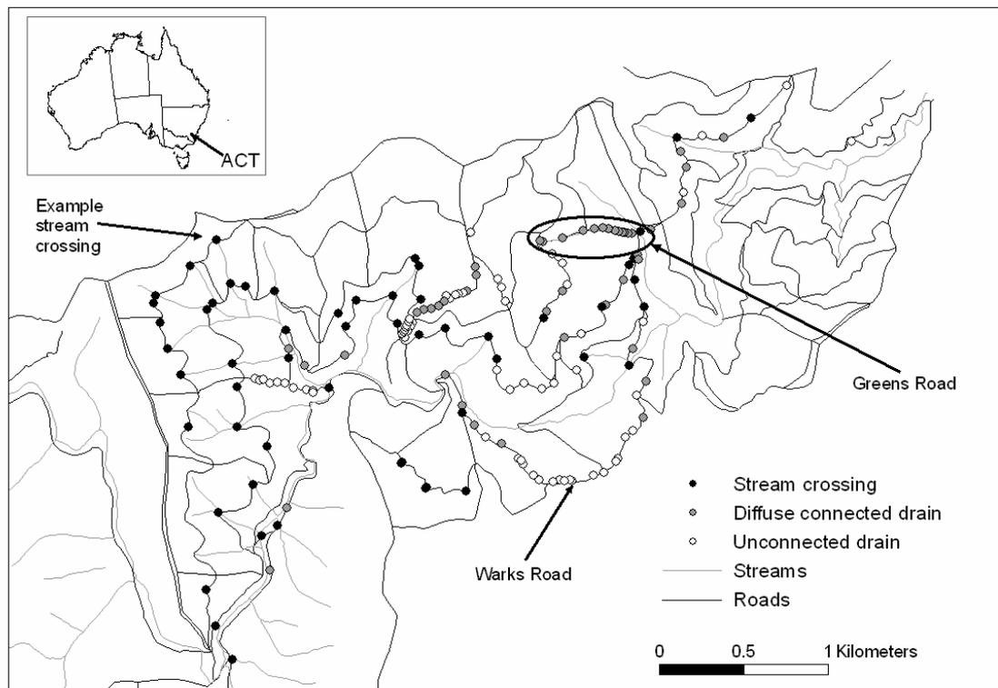
**Fig. 2** The spatial distribution of drains at stream crossings, drains predicted to be connected through diffuse overland flow or to be unconnected during a 10-year event.
