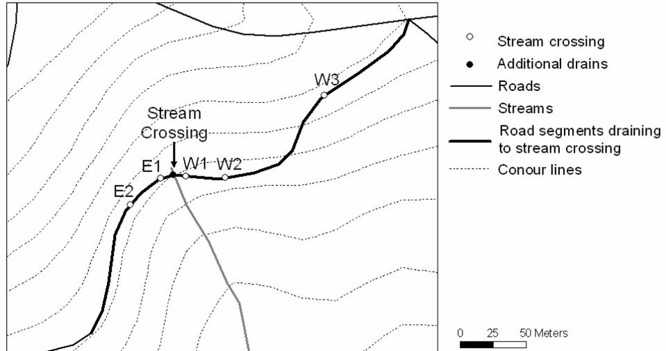
Fig. 3 Proposed location of five additional drains at the example stream crossing.
