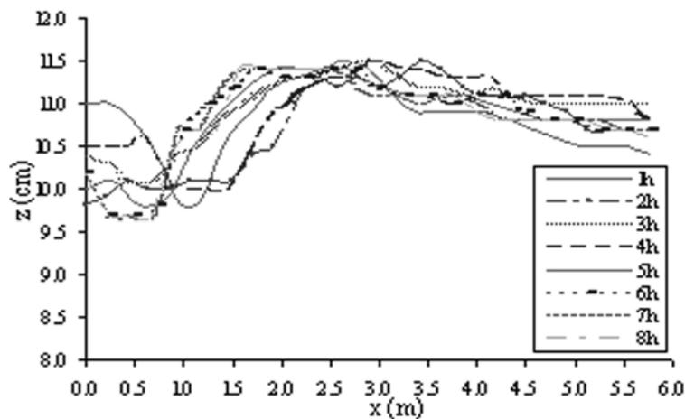
Fig. 3 Longitudinal bed profiles – run 1.
