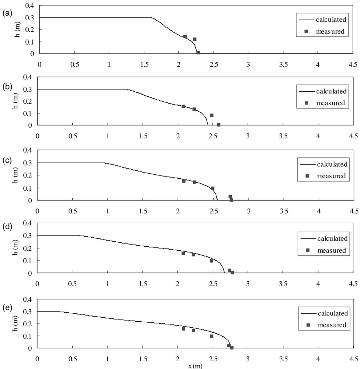
**Fig. 2** Comparison of calculated and measured hyperconcentrated flow depth profiles: (a)  $t = 0.2$  sec; (a)  $t = 0.4$  sec; (a)  $t = 0.6$  sec; (a)  $t = 0.8$  sec; (a)  $t = 1$  sec. (Source of measured data: Komatina & Dordevic, 2004)
