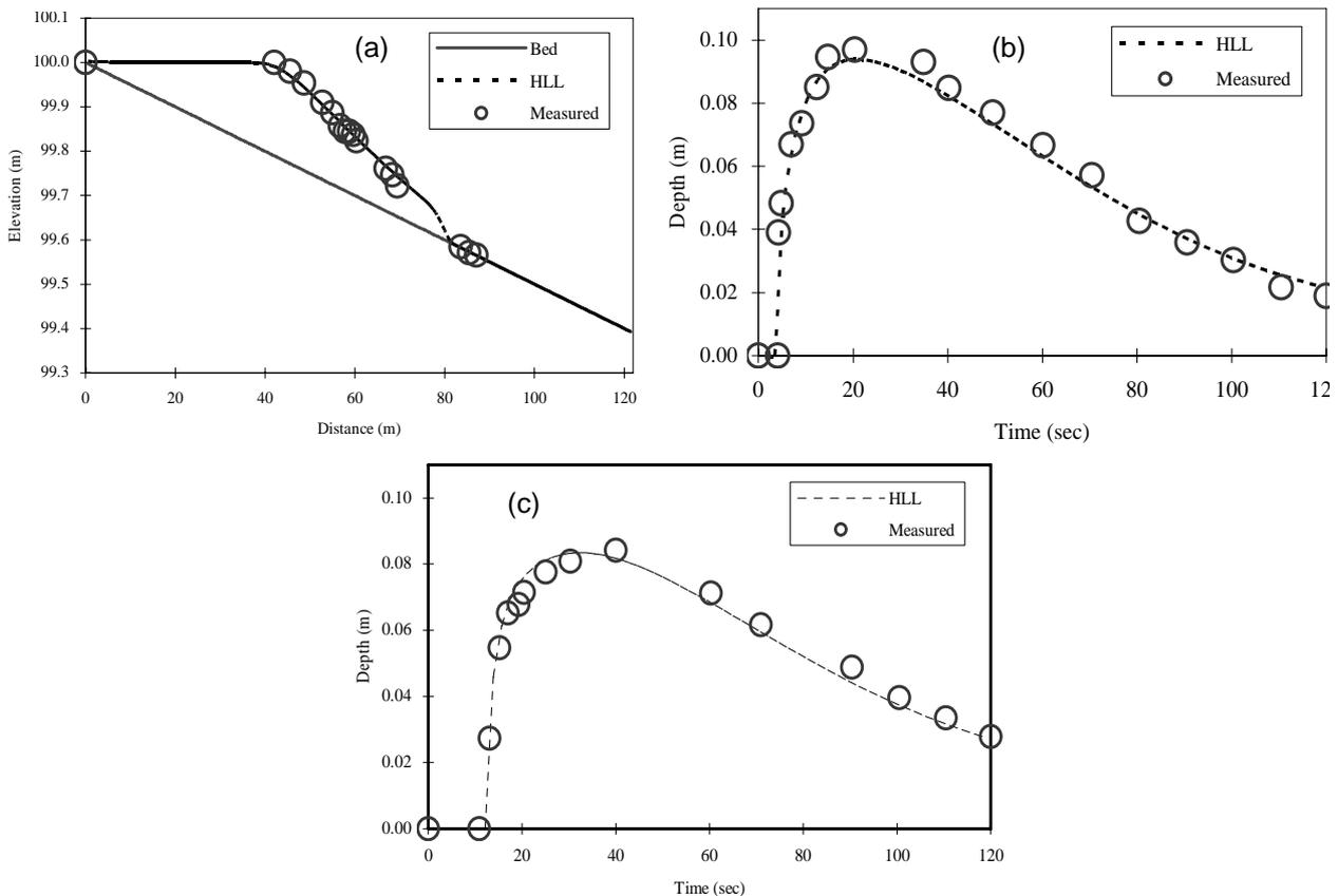
**Fig. 1** Comparison with WES experiment: (a) water surface profile along the channel at  $t = 10$  sec; (b) time evolution of water depth at  $x = 70.1$  m; (c) time evolution of water depth at  $x = 85.4$  m. (Source of measured data: USACE, 1960)
