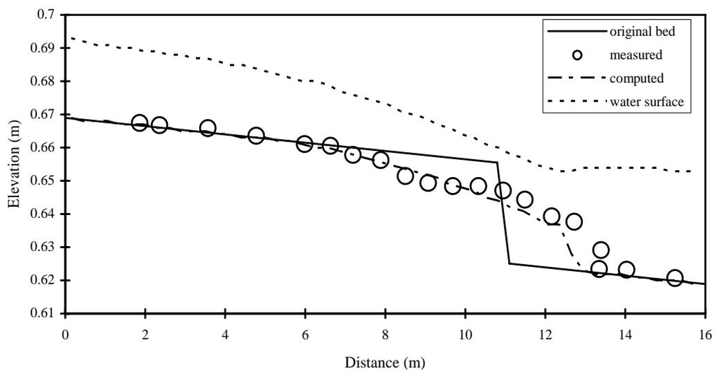
**Fig. 3** Bed level variation due to knickpoint migration. (Source of measured data: Bhallamudi & Chaudhry, 1991).
