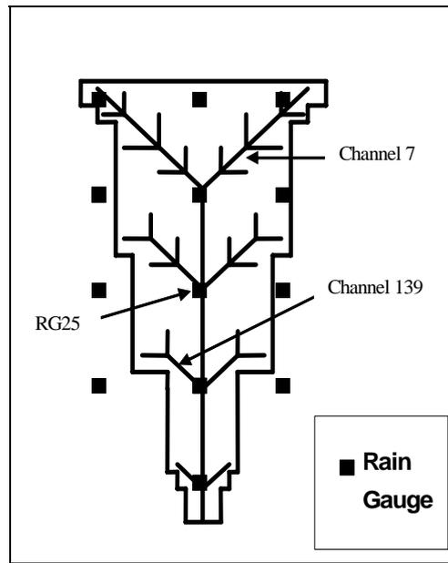
Fig. 1 Basin schematic as seen by the KINEROS2 model.
