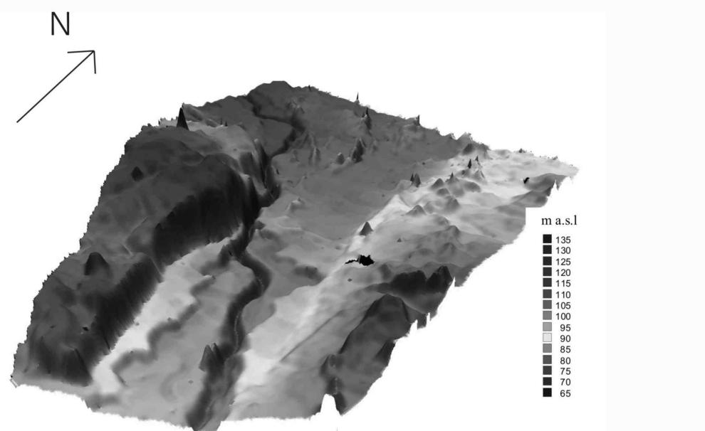
**Fig. 1** Digital elevation model of the Vistula valley in Warsaw showing the city “corset” imposed on the river channel (river flows from south to north).
