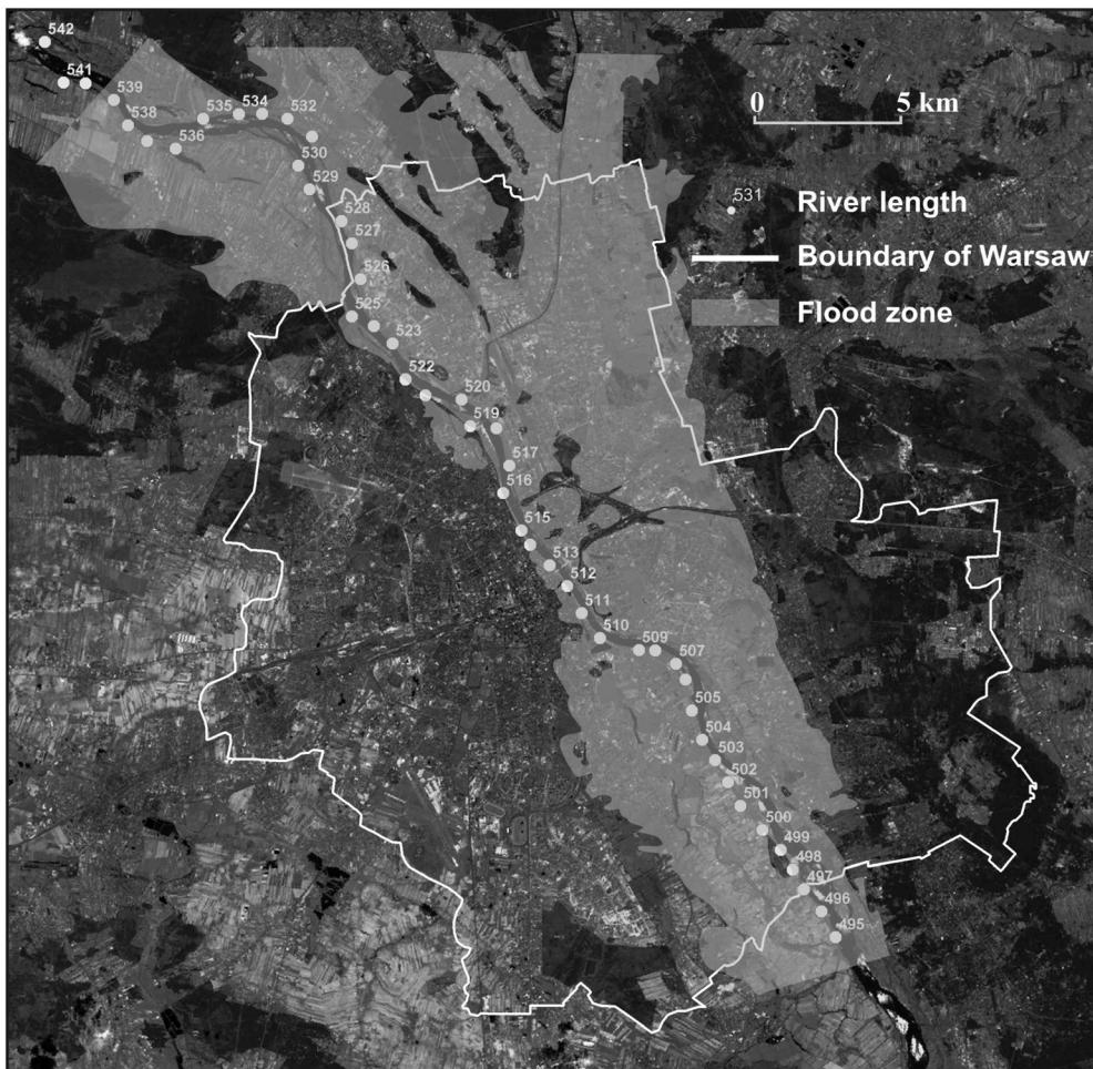
**Fig. 3** Range of Qp0.1% flood zone represented on the background of a Landsat 7 image.
