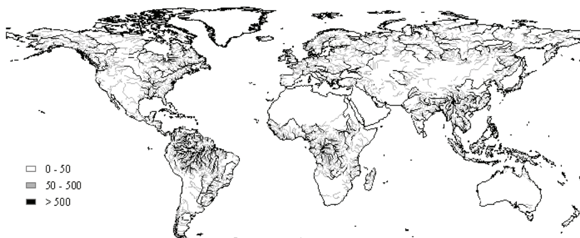
Fig. 1 Predicted river discharge ( \text{m}^3 \text{s}^{-1} ) from the annual composite runoff fields (CRF) data (Fekete et al. , 1999).
