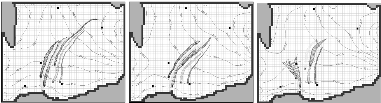
Fig. 5 Extended protection zones obtained with new K heterogeneous distributions and t = 3500 days.
