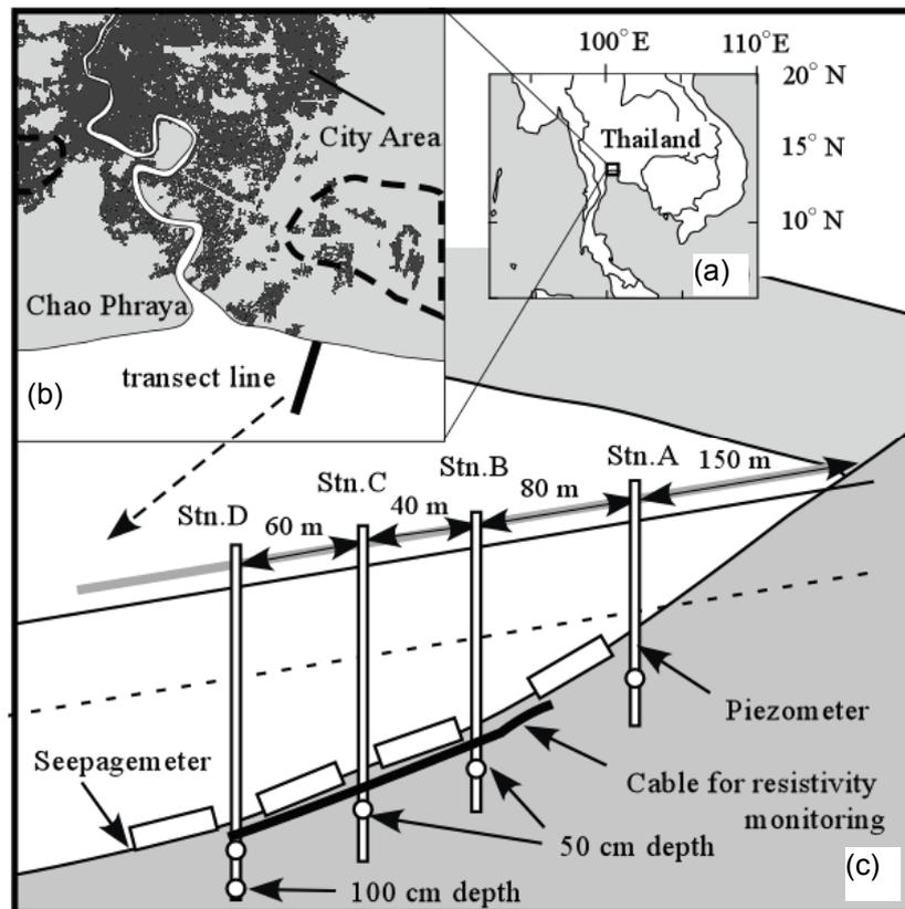
**Fig. 1** Location of study area, and setting design of instruments (piezometers and seepage meters) along the transect line. In (b), enclosed areas with a broken line indicate the areas, where subsidence of over 30 mm/year is currently observed, probably due to groundwater pumping (Phien-wej & Nutalaya, 2006).
