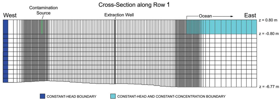
**Fig. 1** Cross-section showing model grid and boundary conditions.
