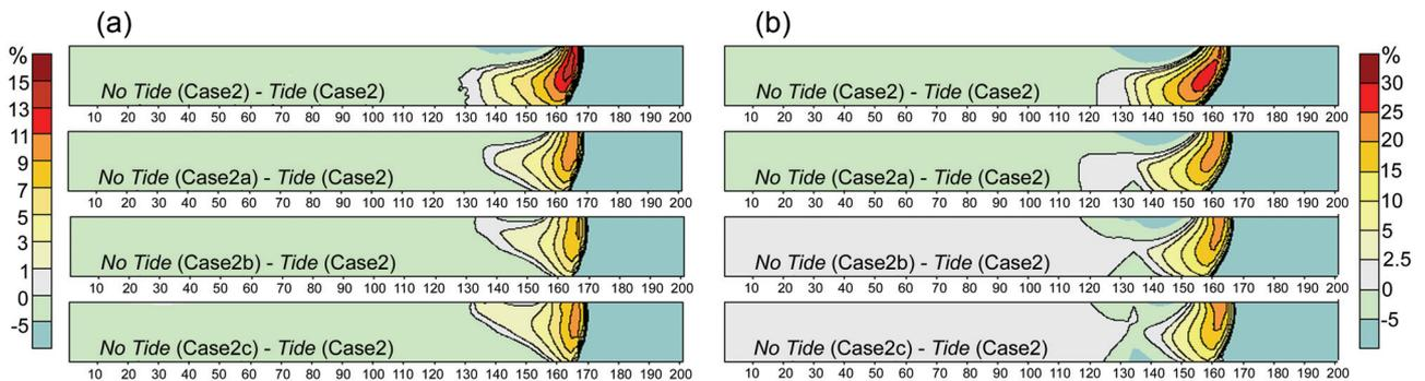
**Fig. 6** Percentage difference in contaminant concentration without (a) and with (b) the extraction well.
