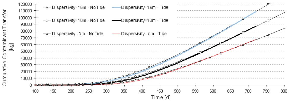
**Fig. 4** Cumulative contaminant transfer from the aquifer to the ocean for the 2-year simulation period, without extraction well.
