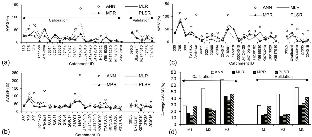
**Fig. 3** The comparison of average width of the interval of simulated flow(AWISF): (a) effect of regional model parameter uncertainty (M1), (b) effect of model parameter uncertainty(M2), (c) effect of combined uncertainty, and (d) average AWISF obtained for various regionalization schemes and various methods (e.g. M1, M2 and M3).
