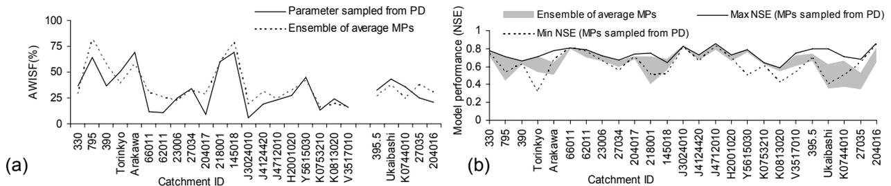
**Fig. 4** Model output for model parameters (MPs) estimated from the regionalization of vectors of MPs and MPs sampled from the posterior distribution: (a) average width of the interval of simulated flow, and (b) range of model performance.
