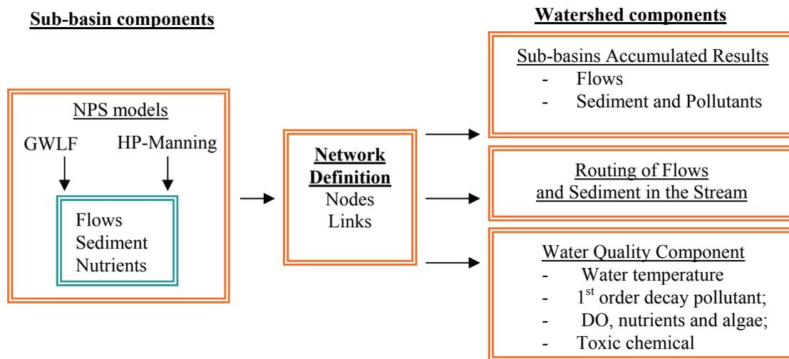
Fig. 1 The interaction of components in WIS during a simulation exercise.
