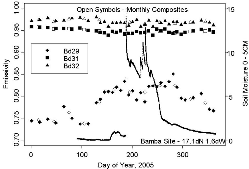
**Fig. 3** Emissivity and soil moisture results for the Bamba, Mali site. The results are for bands 29, 31 and 32 of MODIS whose central wavelengths are 8.55, 11.03 and 12.02  $\mu\text{m}$ . The soil moisture values are for the 0–5 cm soil layer. Note the longitude given in the figure is wrong, it should be 1.3 W.
