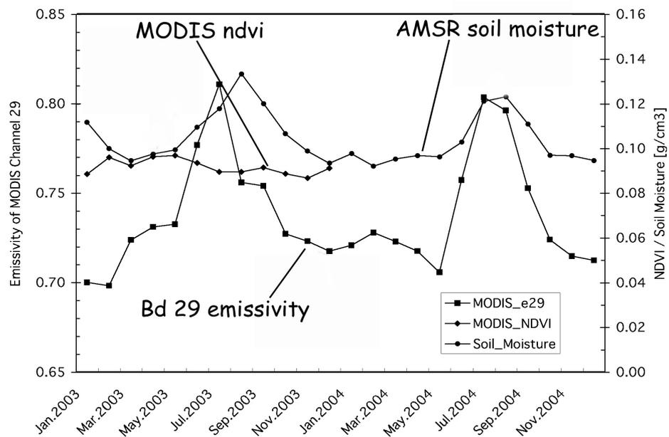
**Fig. 1** Comparison of monthly composites of MODIS band 29 ( $8.55\ \mu\text{m}$ ) emissivity with soil moisture and NDVI for a 2 year period for a location in Mali at  $19^\circ\text{N}$ ,  $3^\circ\text{W}$ .
