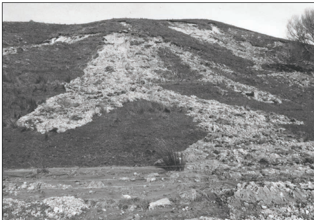
Fig. 2 Most of the failures were flows, with very little material rafted downslope as intact blocks. Note the difference in off-slope delivery associated with this single failure.
