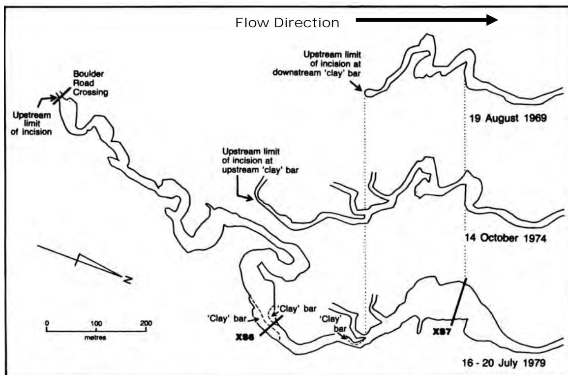
**Fig. 5** Upstream extension of channel incision and widening of Wollombi Brook at Hungry Creek between 1969 and 1979, as determined by field surveys. Location of cross-sections shown in Fig. 2.
