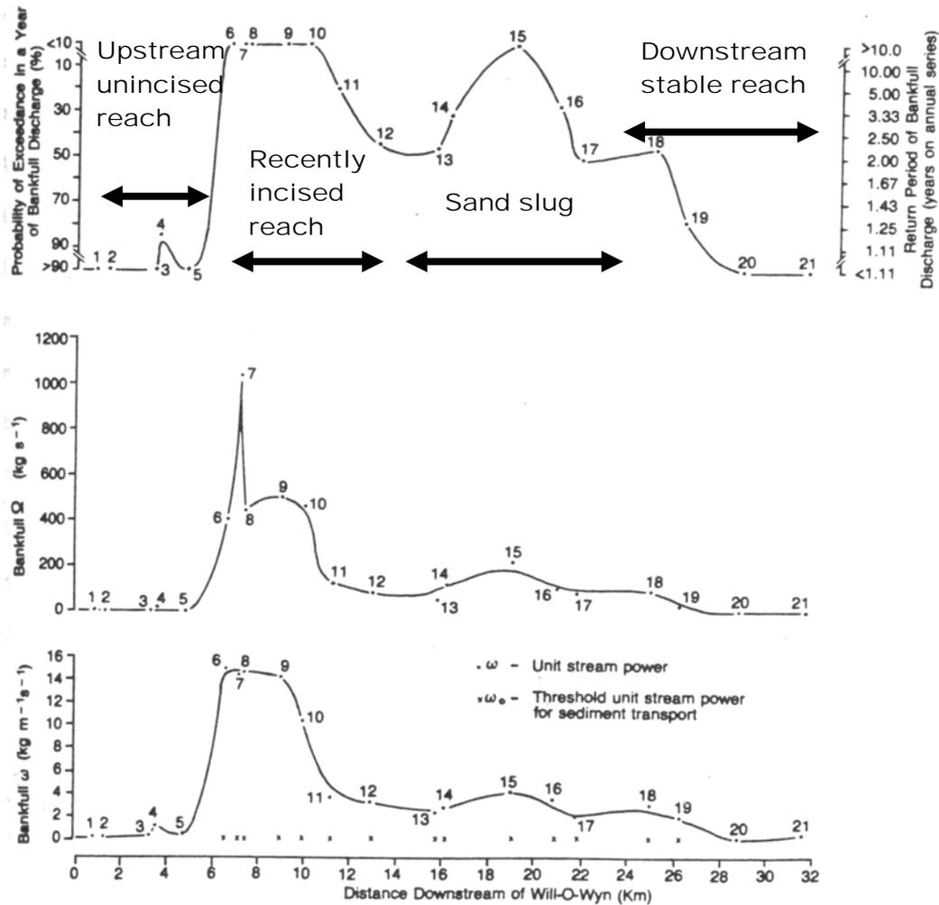
**Fig. 3** Downstream trends in the probability of occurrence of bankfull discharge, and bankfull total, unit and threshold stream power for sediment transport on upper Wollombi Brook. Location of channel cross-sections is shown in Fig. 2.
