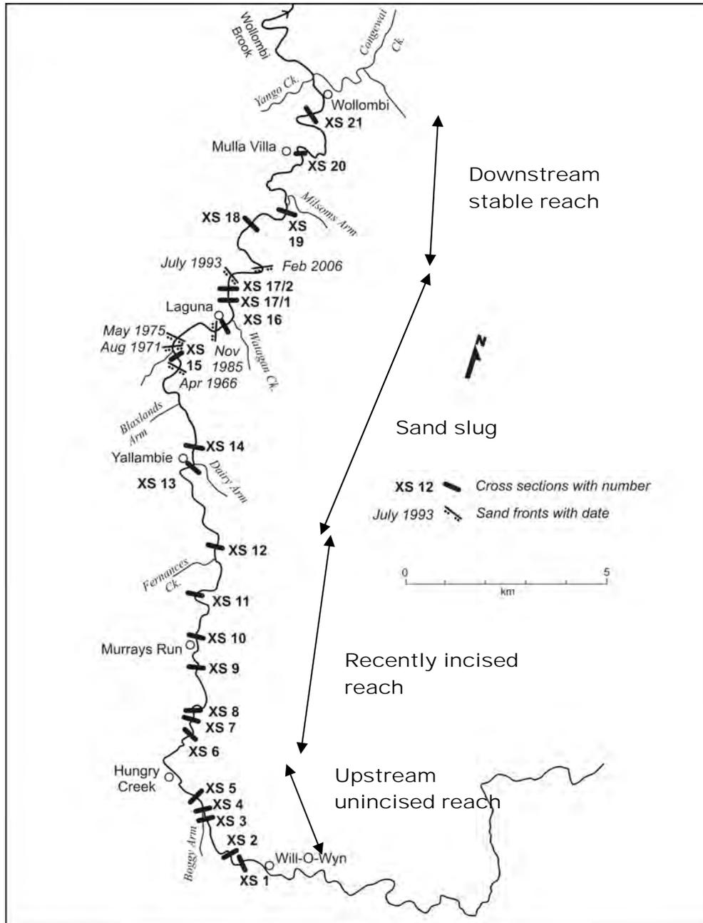
**Fig. 2** Upper Wollombi Brook showing location of channel cross-sections, four channel reaches and downstream movement of the sand front (downstream end of the sand slug/floodout), over time.
