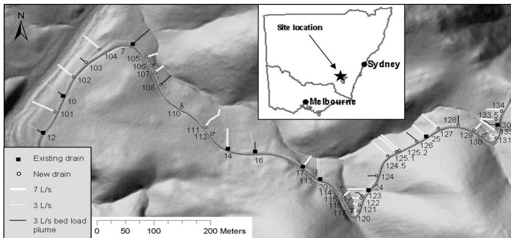
**Fig. 3** DEM with Vanity's Crossing Road along which the pumping experiments were conducted. Site codes with approximate location of flow paths, lengths and bed load plume lengths are indicated.
