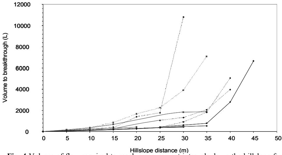
**Fig. 4** Volume of flow required to reach measurement intervals down the hillslope for existing drains. Solid lines indicate flows that connect to streams and dotted lines indicate flows that did not connect.
