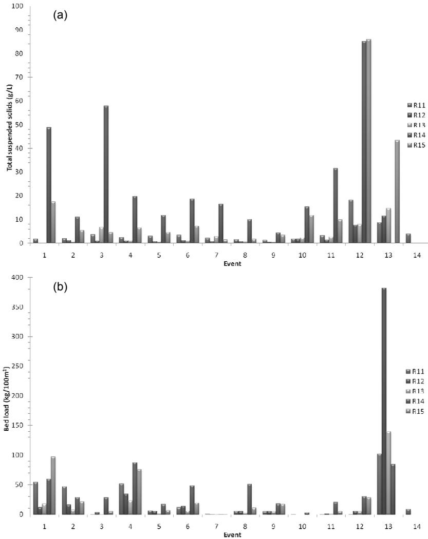
**Fig. 2** (a) Total suspended sediment concentration and (b) bed load per 100 m<sup>2</sup> road contributing area for measured rain events between 20 March 2007 (event #1) and 26 November 2007 (event #14).
