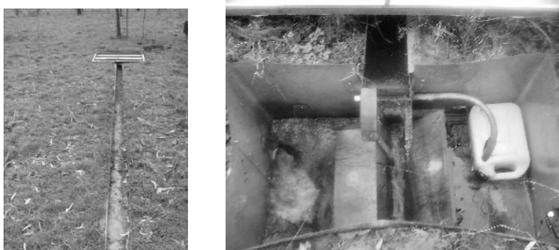
Fig. 2 Runoff trough installed at Meadowvale Station (left). Tipping bucket, logger and sample collection vessel during a runoff event (right).
