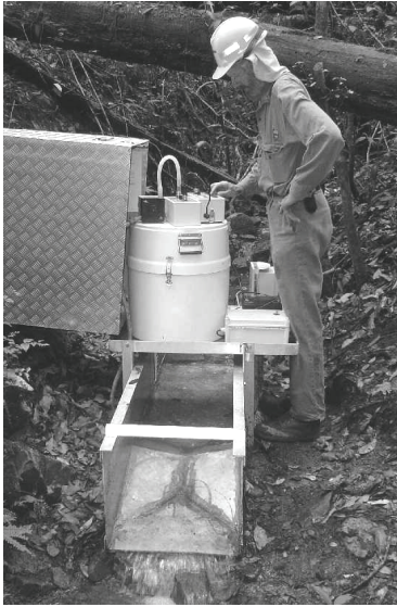
Fig. 1 Flat-v weir at catchment 4 outlet during a runoff event, 25 October 2004.
