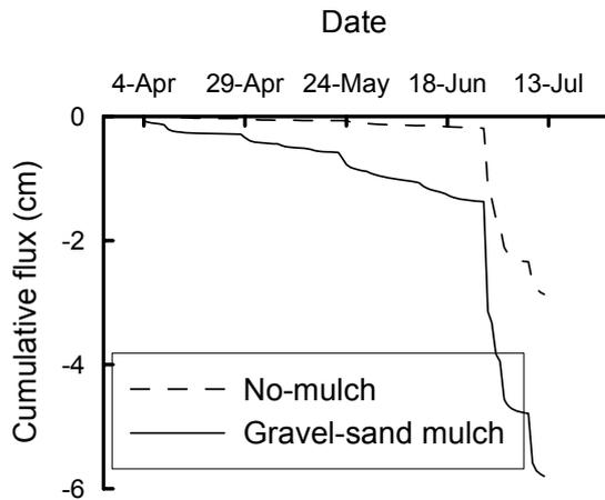
Fig. 3 Cumulative soil water flux at 12 cm depth for the gravel-sand mulch and bare-soil, 4 April–12 July 2001.
