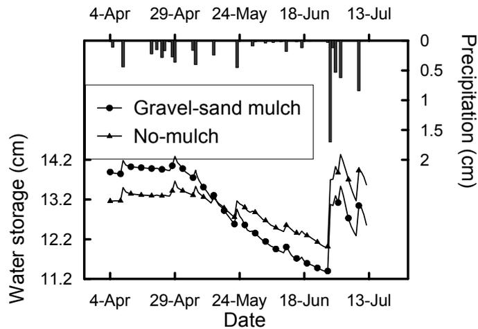
Fig. 2 Measured daily precipitation and simulated water storage of the root zone in the gravel-sand mulch and no-mulch fields, 4 April–12 July 2001.
