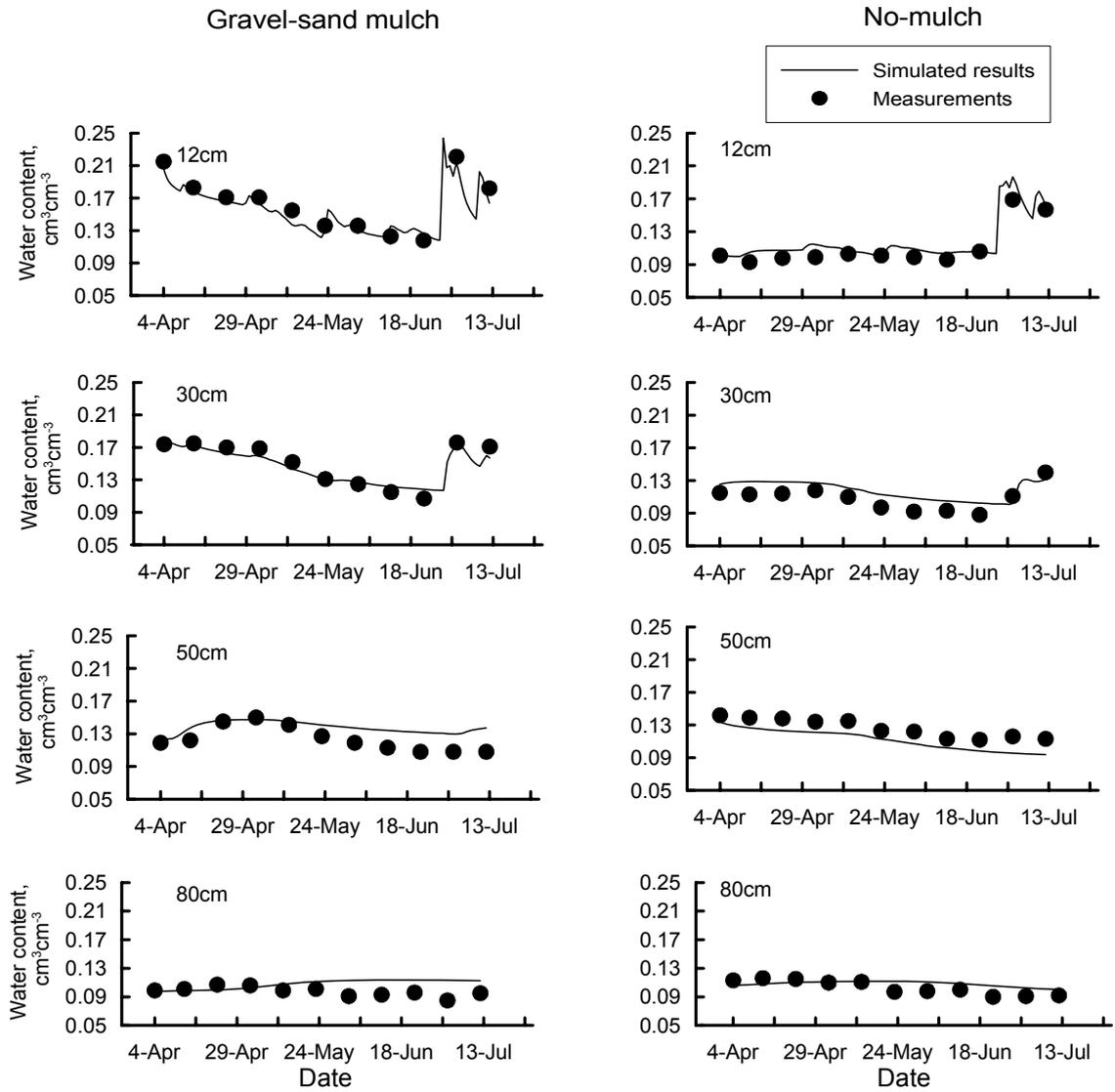
Fig. 1 Observed and simulated water content at 12, 30, 50 and 80 cm depth under the gravel-sand mulch and no-mulch, 4 April–12 July 2001.
