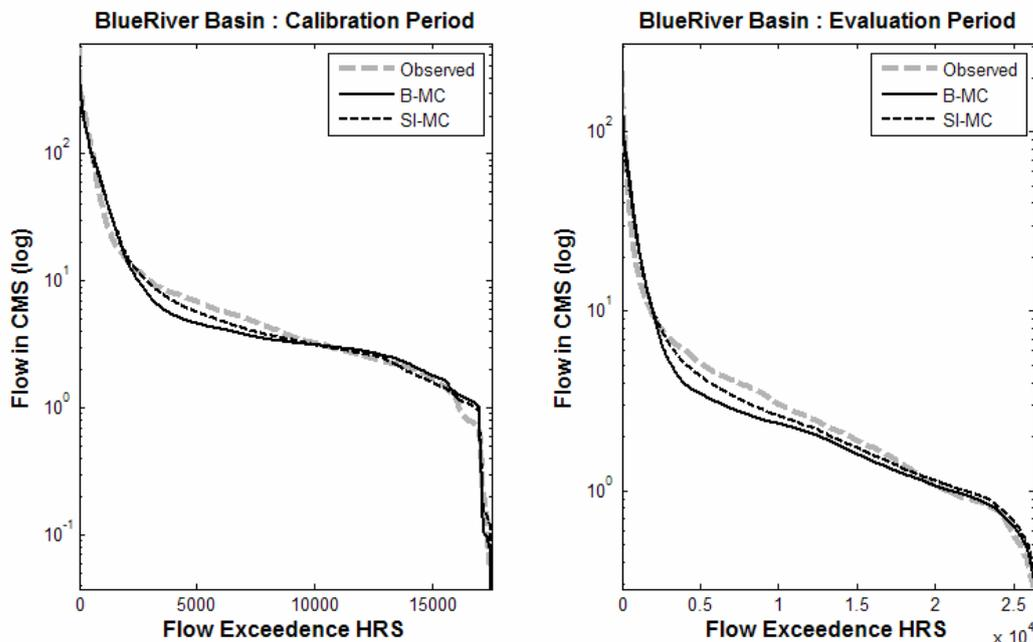
Fig. 3 Simulated and observed flow duration curves comparing B-MC and SI-MC.
